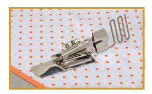
With the wrong side of the fabric facing you, feed the binding strips through the serpentine fabric guide and into the binder.
